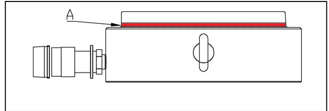
**Figure 4, Maximum Stroke Indicator Line (A)
