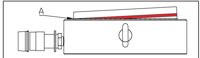
**Figure 5, Maximum Stroke Indicator Line (A)
