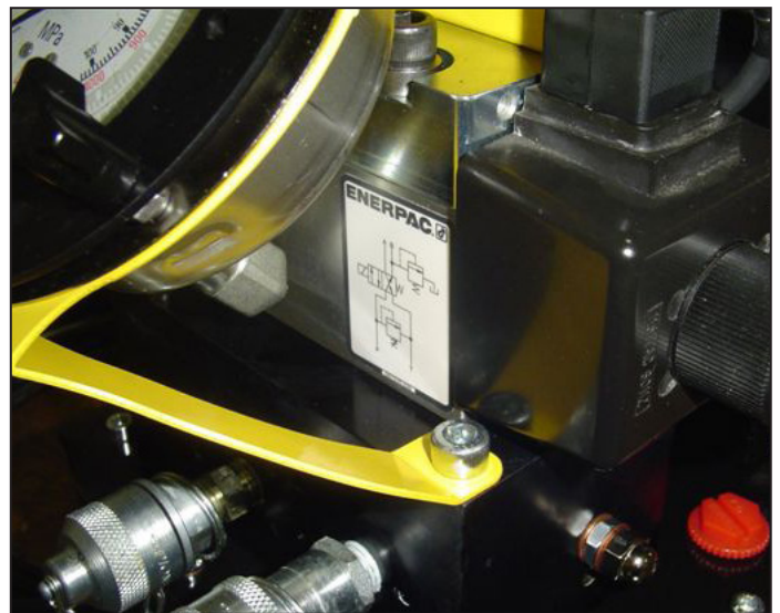
Figure 10, Mounting Screw Securing Gauge Bracket
